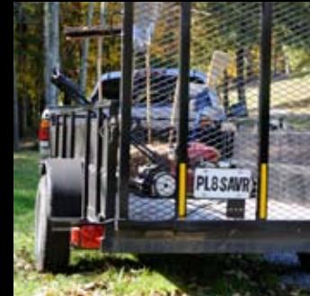
Utility trailers typically have a steel, plastic or rubber license plate mount that attaches below the taillight. This design allows for the plate to be illuminated by the taillight via a clear plastic lens on the bottom of the taillight. This method often limits the clearance of the trailer and causes the license plate damage or even loss due to contact with road or obstacles when maneuvering the trailer.
